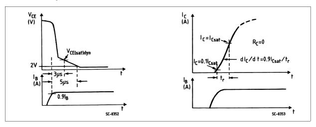
Turn-off SwitchingTest Waveforms (inductive load).
